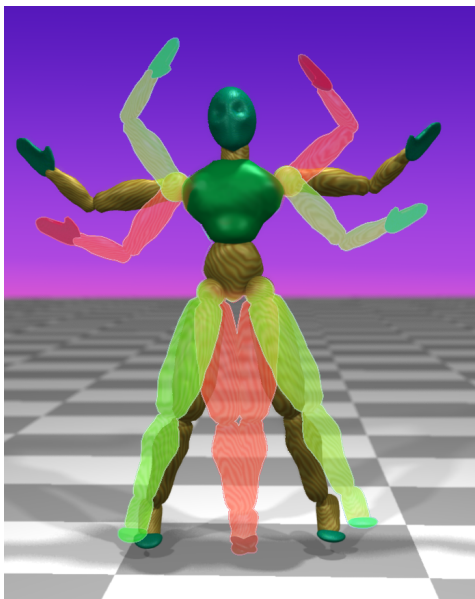
Figure 6: An example of what may happen if the step-length of the Jacobian Transpose method is chosen too high. The motion flips between the green and the red pose, superimposed on the desired result. Step-length in this example was set at 0.05.
