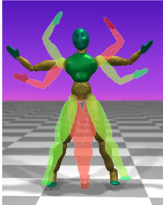
Figure 8: An example of what may happen if the step-length of the Jacobian Transpose method is chosen too high. The motion flips between the green and the red pose, superimposed on the desired result. Step-length in this example was set at 0.05. This example used 5 positional goals and joint limits.
