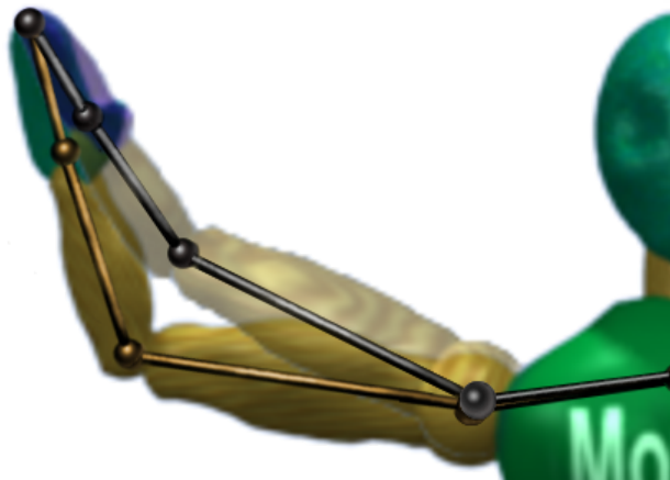
Figure 2: An example of a mathematically correct solution which deviates from the reference due to redundancy. The Ghosted overlay with the grey skeleton is the projected line-search inverse kinematics solution. Notice the large difference on the wrist and elbow and the small but noticeable difference on the shoulder joint. A positional goal was used in this example.
